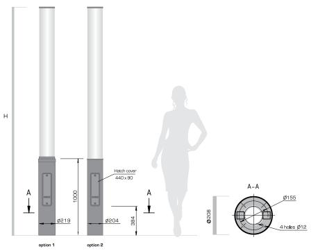
Components Design Included with the product are 2 modifications: light sources (a metalhalide lamp, 1. Steel. fluorescent lamps and LED). 2. Stainless steel. The dome lamp material - opal polycarbonate. Connection Additional information 220 V, 50 Hz Base for installation - FM1T, 3T-1000 or embedded anchors ANK-R (p.206-211). Corrosion protection - HD galvanizing (for option 1). Coating Powder coating in any colour from the standard colour range (p. 213).
