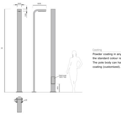
LED The pole is made of aluminium alloy. Available in two modifications: standard and M-modification (with increased power) Connection Additional information 220 V, 50 Hz Base for installation FM3, FM-Powder coating in any colour from TP5 or type 4 (p. 206-211) the standard colour range (p. 213). The max. section of the The pole body can have any colour connected conductors: 16
