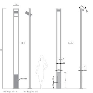
Light sources Pole - steel. Luminaire bracket Metal halide light source or LED. - aluminium alloy.
