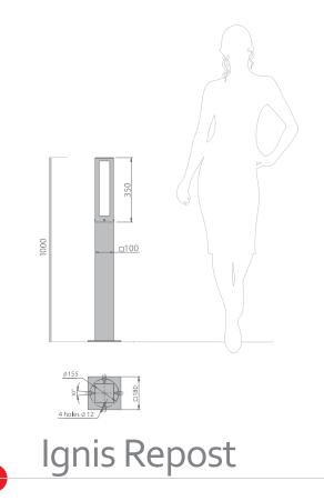
Components Design Included with the product are The body is made of LED light sources. aluminium, the fixtures are made of stainless steel. Diffuser - light-diffusing polycarbonate with UV protection. Height - 1 m (other customized heights are also available). Connection Additional information 220 V, 50 Hz Base FM1T,3T-1000 or embedded anchors ANK-R (p.206-211) are used for bollard installation.
