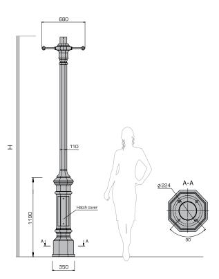
Components The luminaire shall be The pole is made of steel, ordered separately. decorative elements - cast iron. The bore diameter shall be made specifically for each luminaire. Coating Additional information Powder coating in Base for installation anycolourfrom the standard FM6-1500 (p.206-211). colour range (p. 213). Corrosion protection - HD galvanizing (the pole body).
